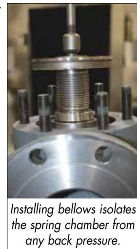
*Installing bellows isolates the spring chamber from any back pressure.*
